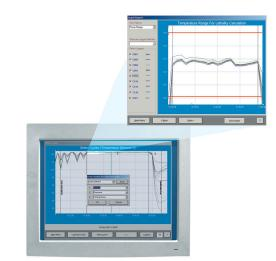
A powerful graphing utility within the system software greatly simplifies process analysis and reporting. Sliding vertical axes allow the operator to flag and define process transition points, eliminating unnecessary reporting and streamlining the review process.
