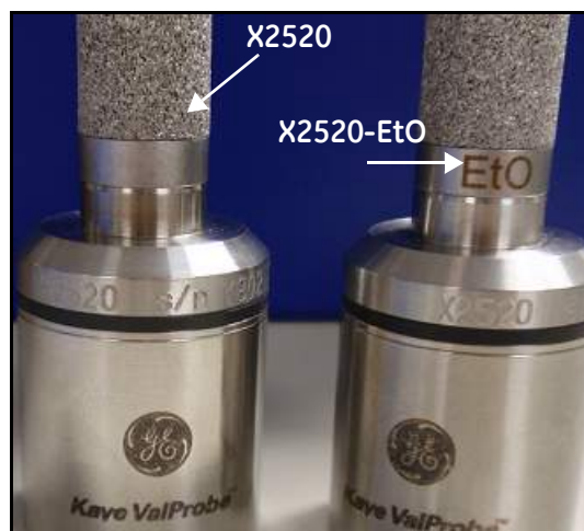
Figure 3: Loggers with and without ETO on Cap
