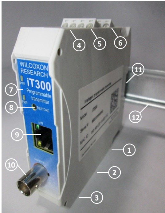
Figure 1 - Major system components
