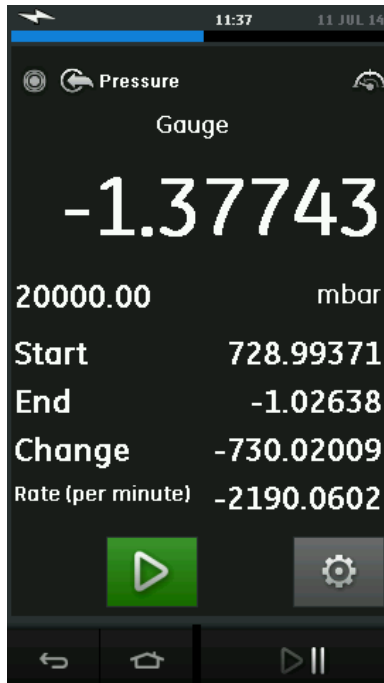
Figure 2-27 Leak Test Example
