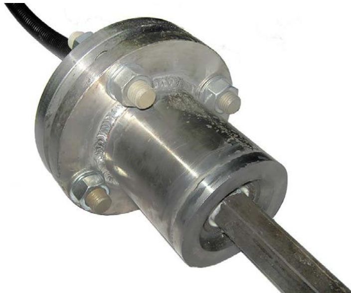
Probe with a front coupling and flange assembly
