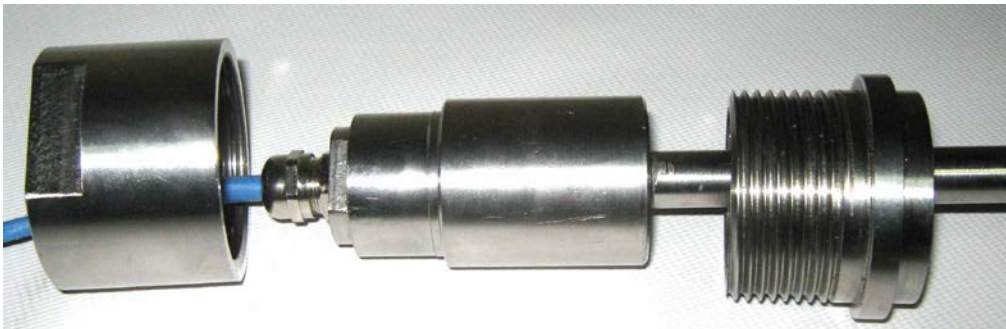
Disassembled front coupling before probe fixing
