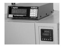
for quick and easy profile programming of RH% and temperature values. You can program up to 256 steps, 40 profile ramp and soak profiles. The DewMaster hygrometer is integrated to the Watlow Controller. Also available at the DewMaster analyzer interface is access to an analog output that may be programmed for RH, Dew Point, or Temperature.
