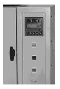
The ELH may be pre-programmed to follow a set of humidity cycles, ramps, soaks or profiles. Programming is done through the Watlow controller shown in the picture to the left. The controller meets the requirements of the most demanding ramp soak controller processing applications. Easy to set up and operate, the controller's programming features and proven performance capabilities are ideally suited for the humidity control applications.
